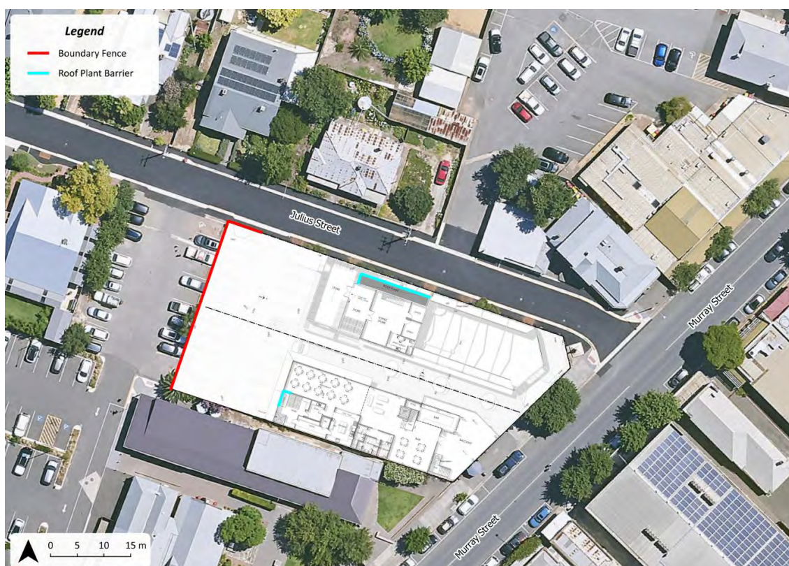
Figure 2: Recommended Barrier Locations
